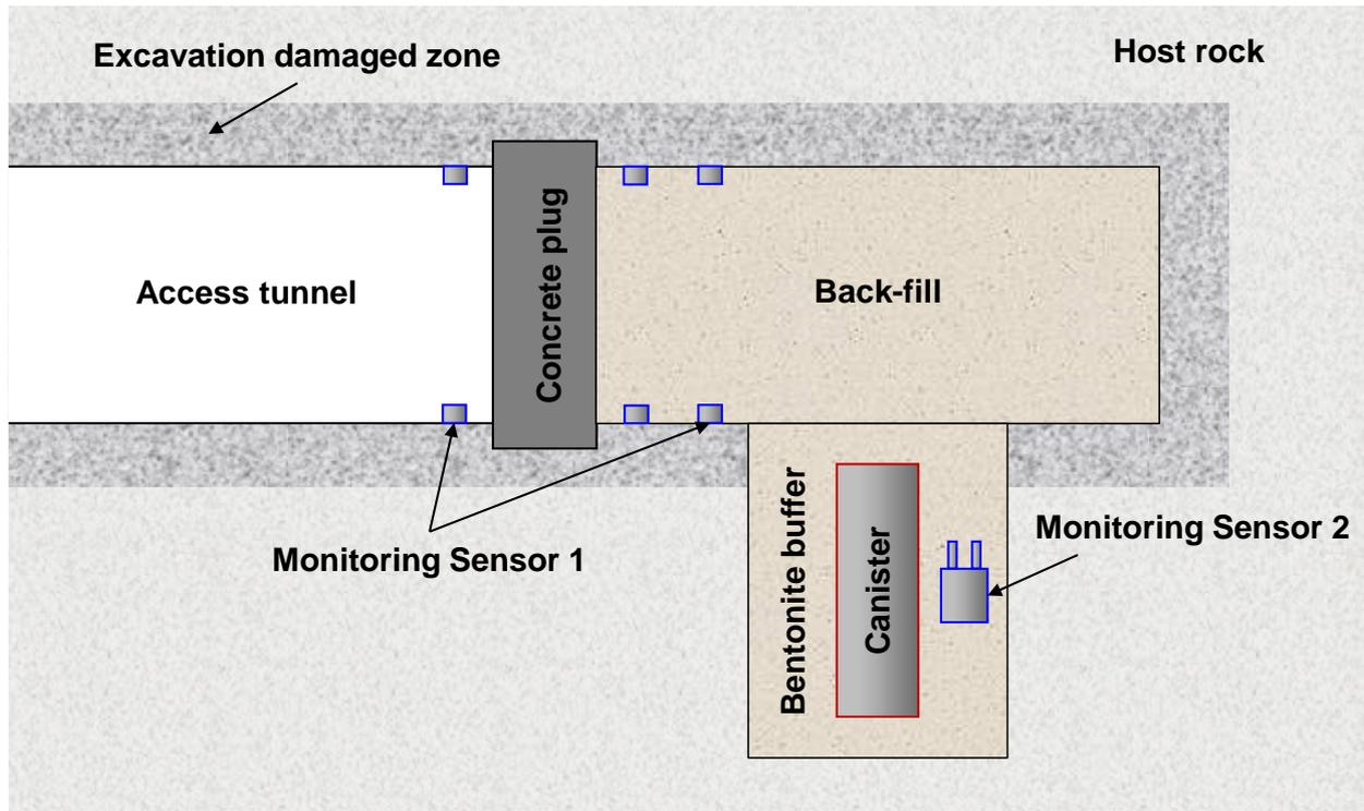
Fig. 2 Locations of the sensors at HLW repository
