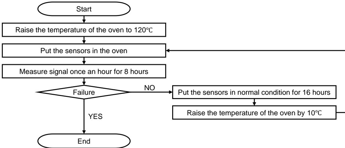
Fig. 4 Flow chart of the experiment
