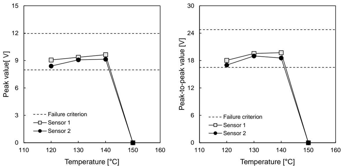
Fig. 6 Peak value and Peak-to-peak value according to temperature
