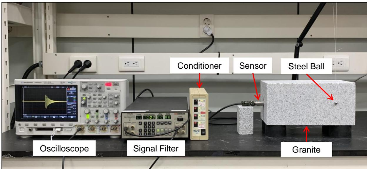
Fig. 5 Experimental equipment
