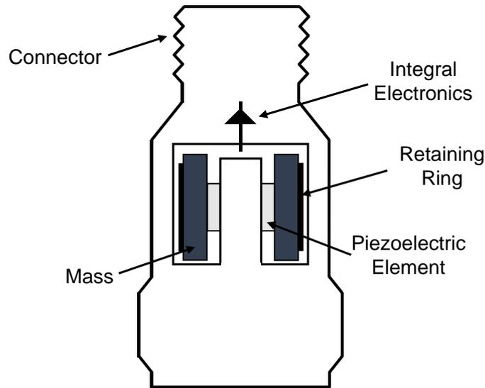
Fig. 3 Typical Industrial Shear Mode Accelerometer
